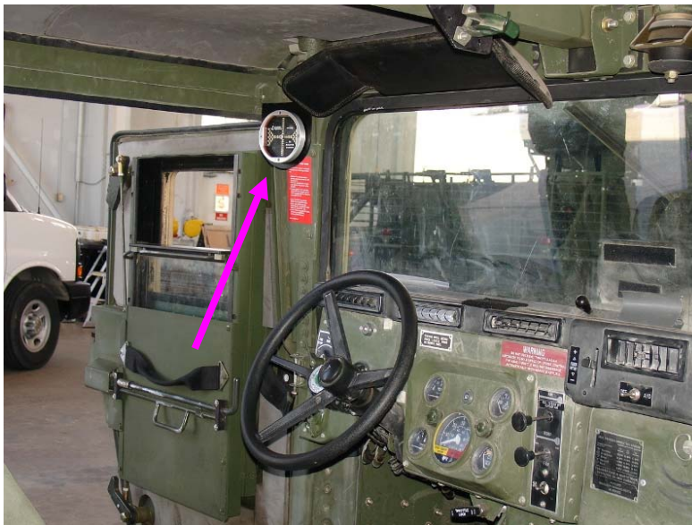
Figure 4. Driver's Display Mounted in Top Left Corner of M1114 Cab
