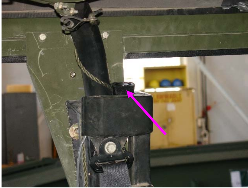
Figure 5. Warning Siren Mounted Above the Driver's Seatbelt Shoulder Mount)
