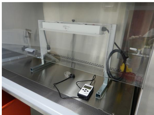
Figure 1. Lind Equipment UV-C Device in CL3 BSC.
